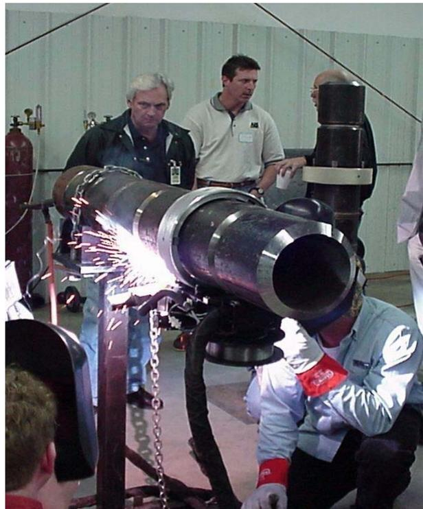
Figure 2. Demonstration of automatic orbital welding of a fixed 5G (double up) P91 pipe using Supercore F91 FCW<sup>\*</sup>
