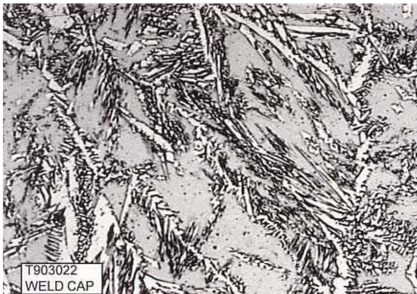
Figure 2. Typical microstructure of weld metal of Supercore 2205P, \times 400
