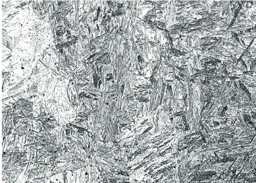
**Figure 4: Typical P91 weld metal microstructure**
