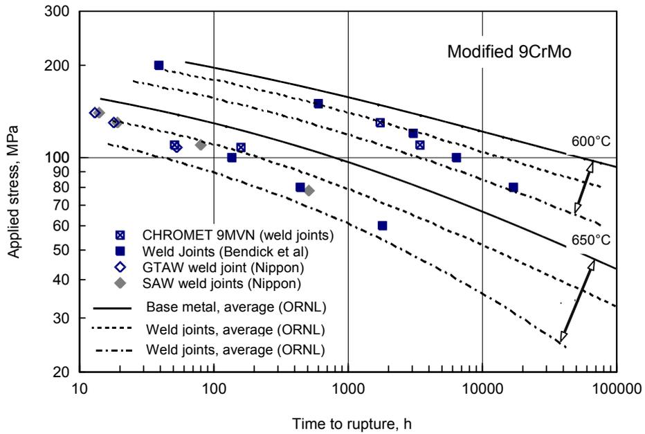
**Figure 2. Creep properties of modified 9CrMo material weldments**
