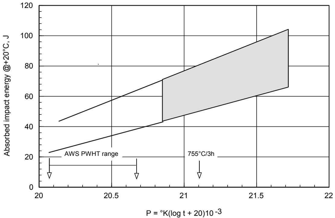
**Figure 4. The effect of PWHT temperature and time on weld metal toughness**
