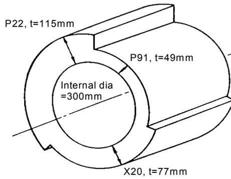
**Figure 1. Comparison of required wall thicknesses for equivalent service. (Temperature 600°C, pressure 30MPa, 100,000h life)**
