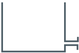
Figure 21 Side outlet, flush—good
