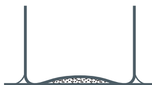
Figure 17 Concave bottom, rounded corners—good inside, good outside, fatigue resistant
