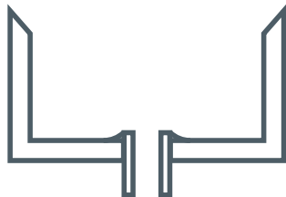
Figure 20 Centre outlet, above bottom—poor
