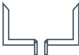
Figure 24 Centre outlet, recessed, sloped—best
