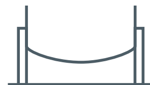
Figure 18 Dished head—best inside, best outside, fatigue resistant
