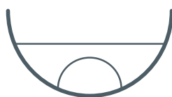
Figure 38 Heat exchanger, baffle cut-out—good
