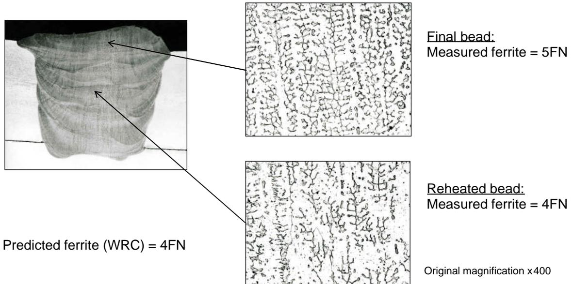
**Figure 10 Microstructure of a vertical-up weld deposited with Supercore 308LCF flux cored wire using Ar-20%CO<sub>2</sub>, in 12.5mm (0.5inch) 304L plate**
