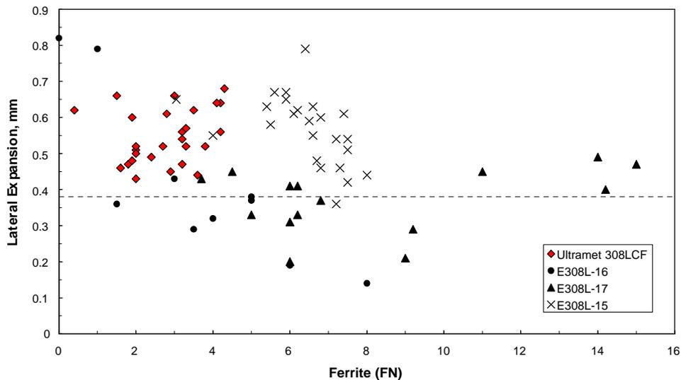
**Figure 5 Weld ferrite versus lateral expansion for 308L SMAW electrodes at  $-196^{\circ}\text{C}$  ( $-320^{\circ}\text{F}$ ). Note the superiority of Ultramet 308LCF, a specially designed rutile electrode, compared with conventional rutile E308L-16/17 types**
