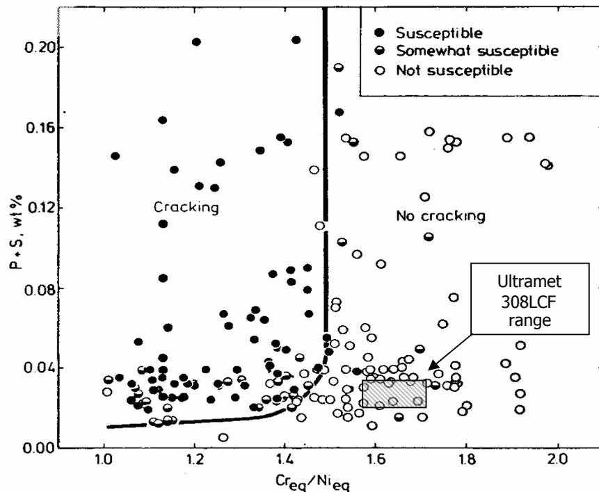
**Figure 6** Suutala diagram [17] with the Ultramet 308LCF SMAW electrode composition range superimposed. The Ultramet 308LCF composition range is well in the “no cracking” region of the Suutala diagram.
