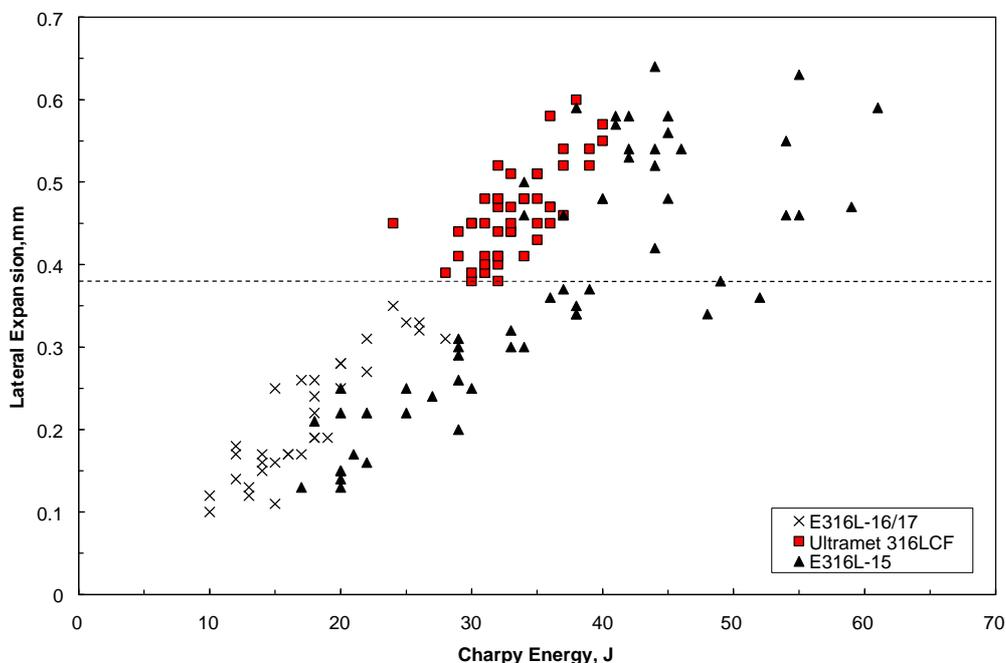
**Figure 7** All-weld metal -196°C (-320°F) impact properties for 316L SMAW electrodes showing the effect of different coating types. (Data plotted are for individual Charpy specimens)
