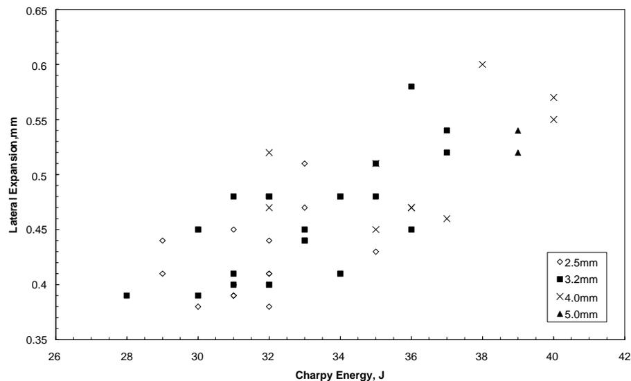
**Figure 11 All-weld metal impact energy versus lateral expansion at -196°C (-320°F) for Ultramet 316LCF SMAW electrode. (Data plotted is for individual Charpy specimens)**
