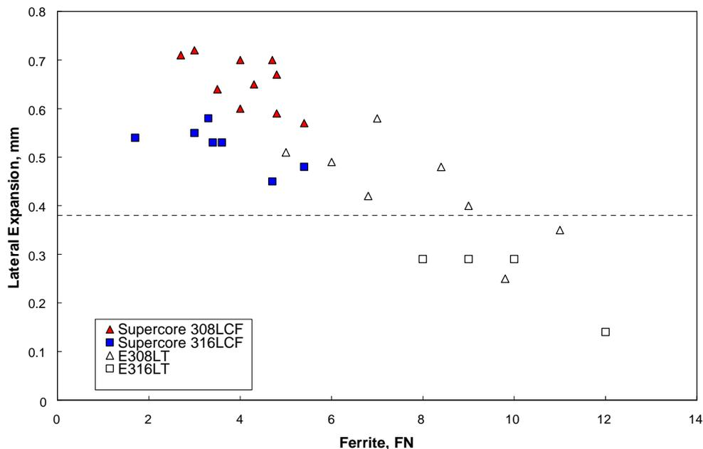
**Figure 8** Effect of weld metal ferrite on lateral expansion at  $-196^{\circ}\text{C}$  ( $-320^{\circ}\text{F}$ ) for flux cored wires. The superiority of the specially designed 'CF' wires is clearly shown. (Data plotted are based on average lateral expansion from a set of Charpy specimens)
