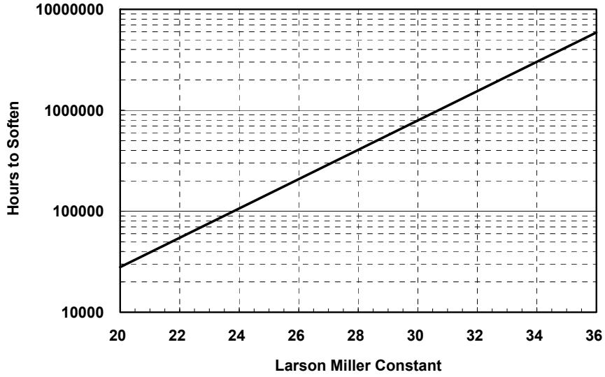
Figure 8 Estimated duration of alloy strength start softening vs. Larson-Miller constant (Operating temperature: 615°C; tempering temperature: 760°C)
