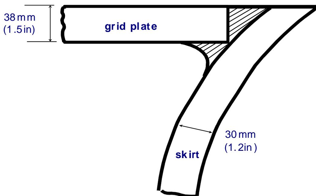
**Figure 4a:** Site butt weld between 38mm (1.5in) grid plate and 30mm (1.2in) thick skirt plates
