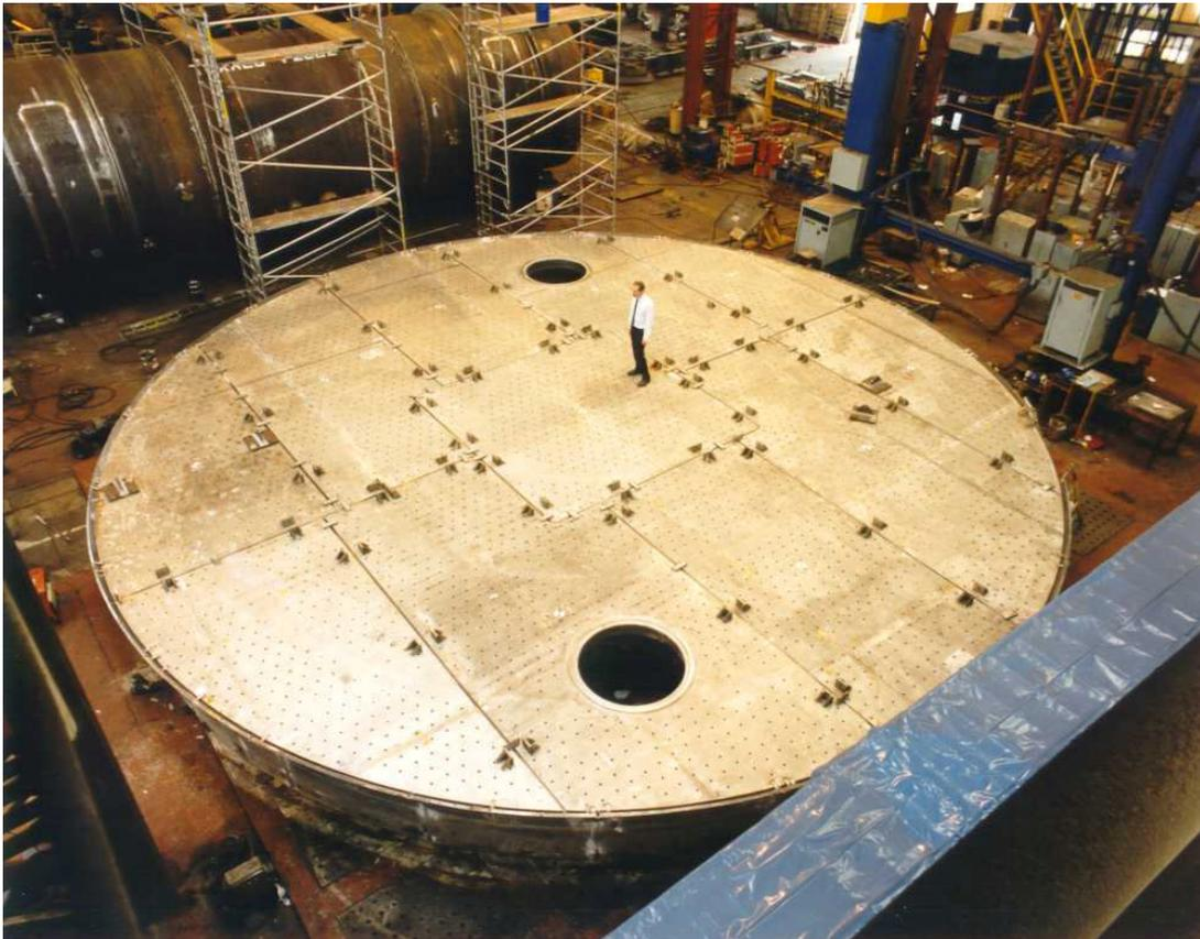
**Figure 1:** Catalyst support grid trial assembly in the fabrication shop showing section layout and welded joints to be completed on site.
