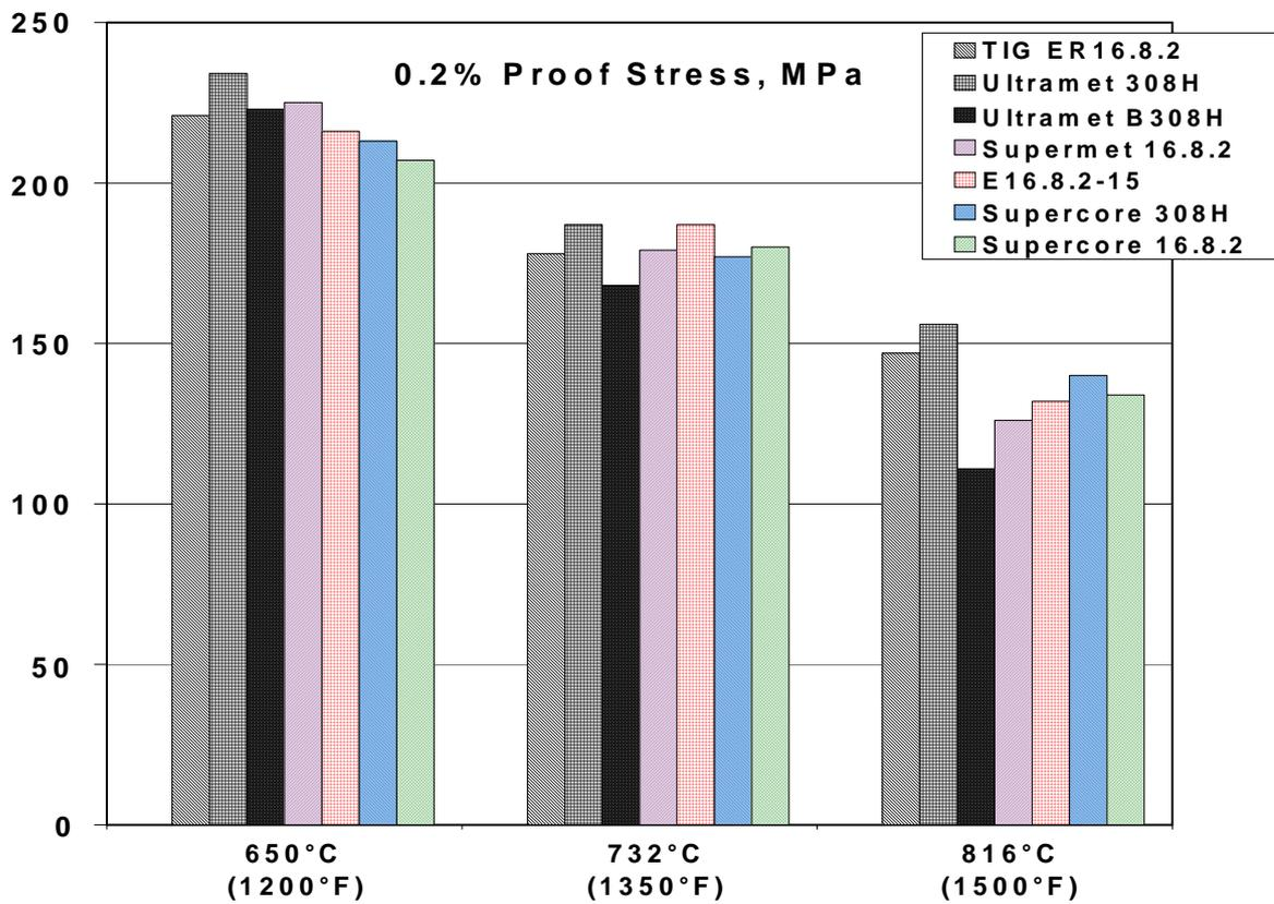
**Figure 6: Elevated temperature strength and ductility properties of 308H and 16.8.2 from all-weld metal hot tensile tests**
