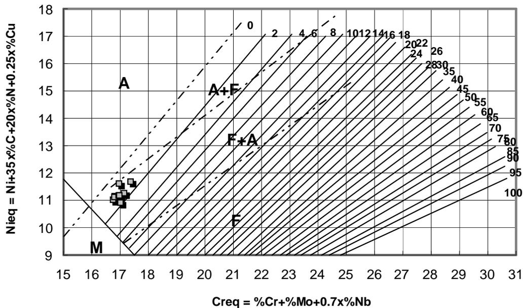
**Figure 5b: Extended WRC-92 diagram showing the position of 16-8-2 FCW weld metal**
