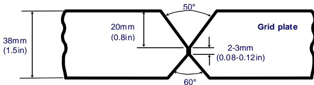
**Figure 3a:** Shop pre-fabricated butt welds in 38mm (1.5in) grid plate
