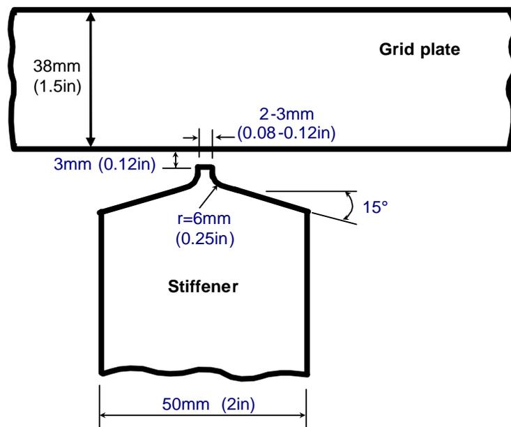
**Figure 3b:** Shop pre-fabricated butt welds between 38mm (1.5in) grid plate and 50mm (2in) thick stiffener
