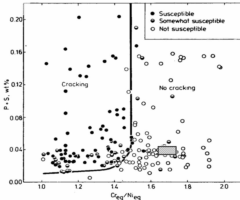
**Figure 5a: Suutala Diagram showing position of 16-8-2 FCW weld metal in the "no cracking" region**
