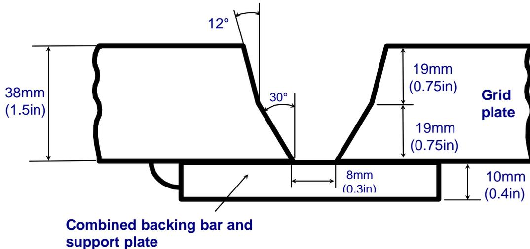
**Figure 4b: Site butt welds in 38mm (1.5in) grid plate with access from the top side only**
