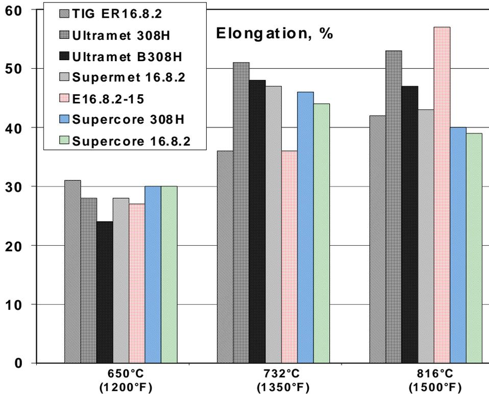
**Figure 6 continued: Elevated temperature strength and ductility properties of 308H and 16.8.2 from all-weld metal hot tensile tests**
