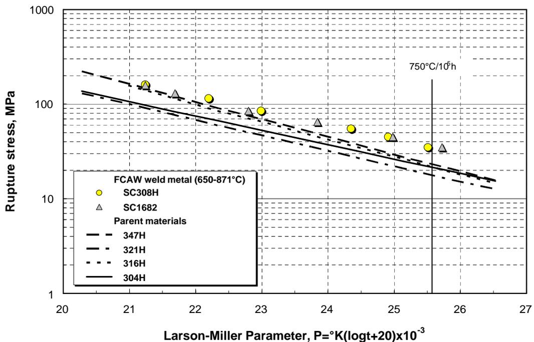
**Figure 7: Larson Miller plot of stress-rupture data obtained for Supercore 308H and Supercore 16.8.2 FCAW weld metal compared with minimum 10<sup>5</sup>h rupture stress for relevant austenitic 3xxH parent materials (from ASTM DS 5S2)**
