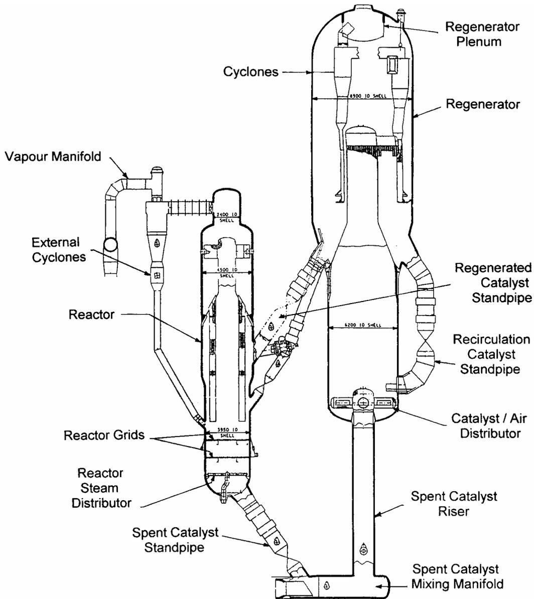
**Figure 2: Recent (1998) design for cat cracker showing all major components. Note that catalyst recovery cyclones are external on the small reactor vessel (left) and internal on the large regenerator vessel (right).**
