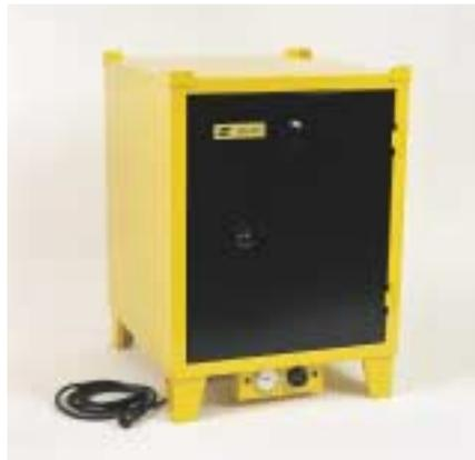
The SK 40 is a dry-storage cabinet with four removable shelves for storing electrodes. The electrodes should be stored without packing. The cabinet is equipped with a thermometer, thermostat and control lamp.
