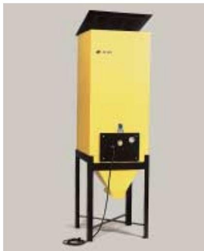
Suitable flux quantities depend on the design and ventilation of the oven, but the height of the flux layer should not exceed 50 mm. Rebaked flux should be stored at  $150 \pm 25^{\circ}\text{C}$  until use.
