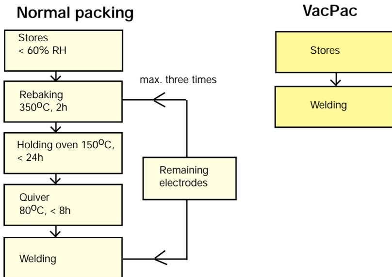
Fig 2. Comparison of procedures for guaranteeing dry electrodes in a workshop between normal packaging and VacPac™.
