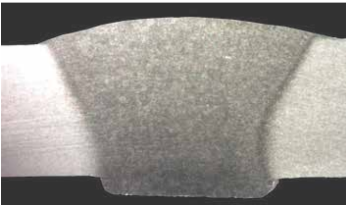
1 Pass - 1.6 mm 5356 - approximately 22 ipm travel speed 23.0 V; 342 ipm wire feed speed
