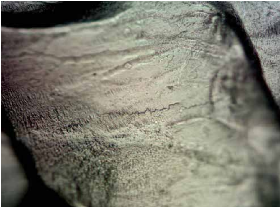
Micro-cracks are potential crack starters in aluminum welds.
