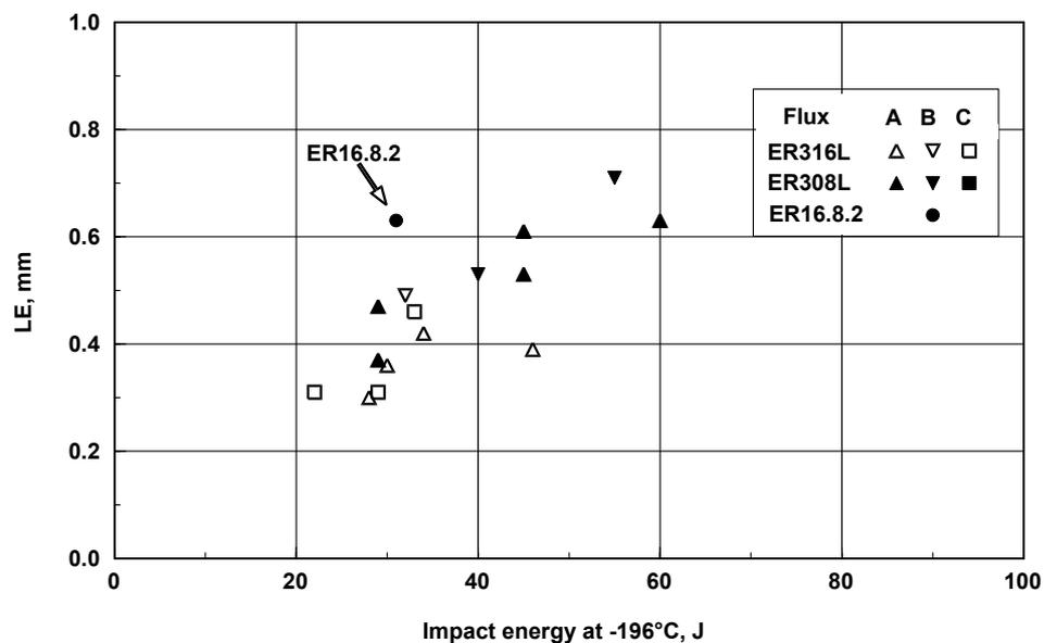
In view of the useful cryogenic properties of 16.8.2, which arise from its relative safety at low FN levels coupled with low microsegregation and embrittlement tendency, it is surprising that no reference to cryogenic applications is given in a recent review<sup>[10]</sup> or in the appendix to AWS A5.4.
