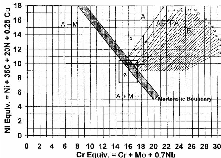
Weld metals of 16.8.2 type were not included in the WRC ferrite database and consequently the current WRC-1992 diagram cuts off at 17Cr eq. Fortunately, extension of the WRC iso-ferrite lines provides very satisfactory agreement between prediction and measurement. The ferrite lines are extended to Kotecki's martensite boundary in Figure 2.
