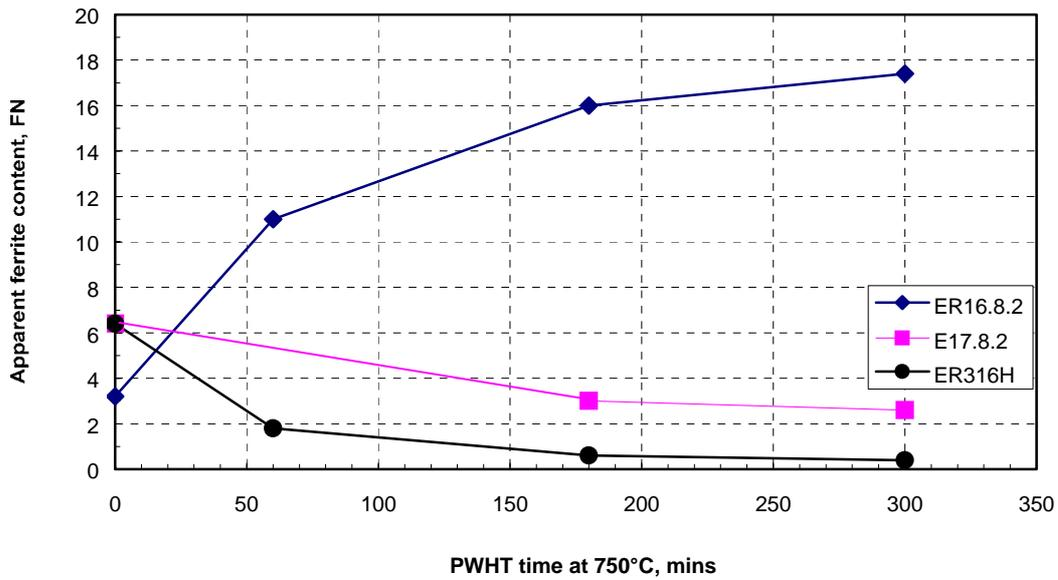
Figure 3: Effect of PWHT at 750 °C on weld metal ferrite (magnetic response) in GTAW ER16-8-2 compared with ER316H and SMAW 17.8.2
