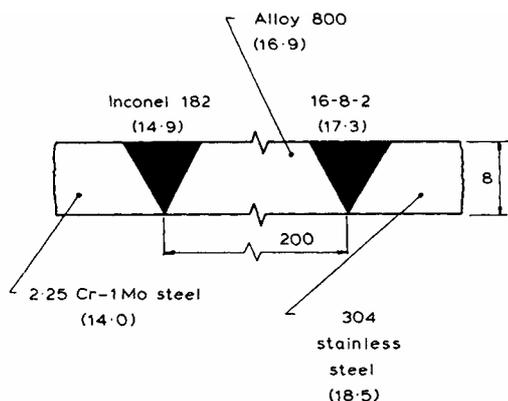
Figure 8: Use of 16.8.2 weld metal for transition joint in prototype fast breeder reactor. Thermal expansion coefficients are shown in brackets [19]
