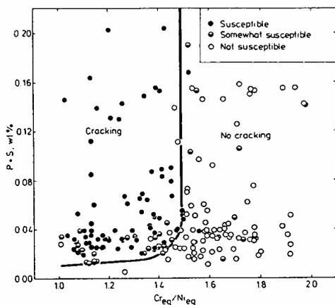
Figure 5: Suutala diagram [10] showing crack / no crack boundary at  $C_{req}:N_{ieq}$  ratio of about 1.5  $C_{req} = Cr + 1.5Si + 1.37Mo$ ,  $N_{ieq} = Ni + 0.31Mn + 22C + 14.2N$
