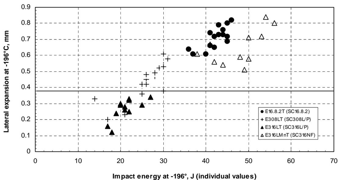
Figure 7: Relationship between Charpy impact energy and lateral expansion of E16.8.2T, E308LT, E316LT and E316LMnT FCAW weld metals at -196 °C
