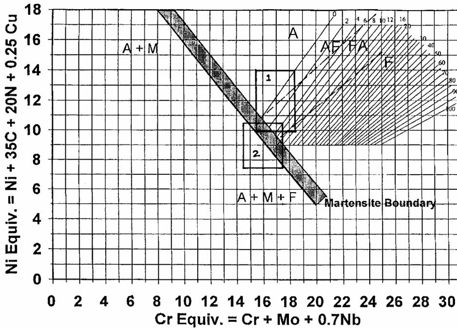
Figure 2: WRC diagram showing location of 16.8.2 weld metal (area 1) and the same with carbon and chromium removed from the matrix as  $M_{23}C_6$  (area 2)
