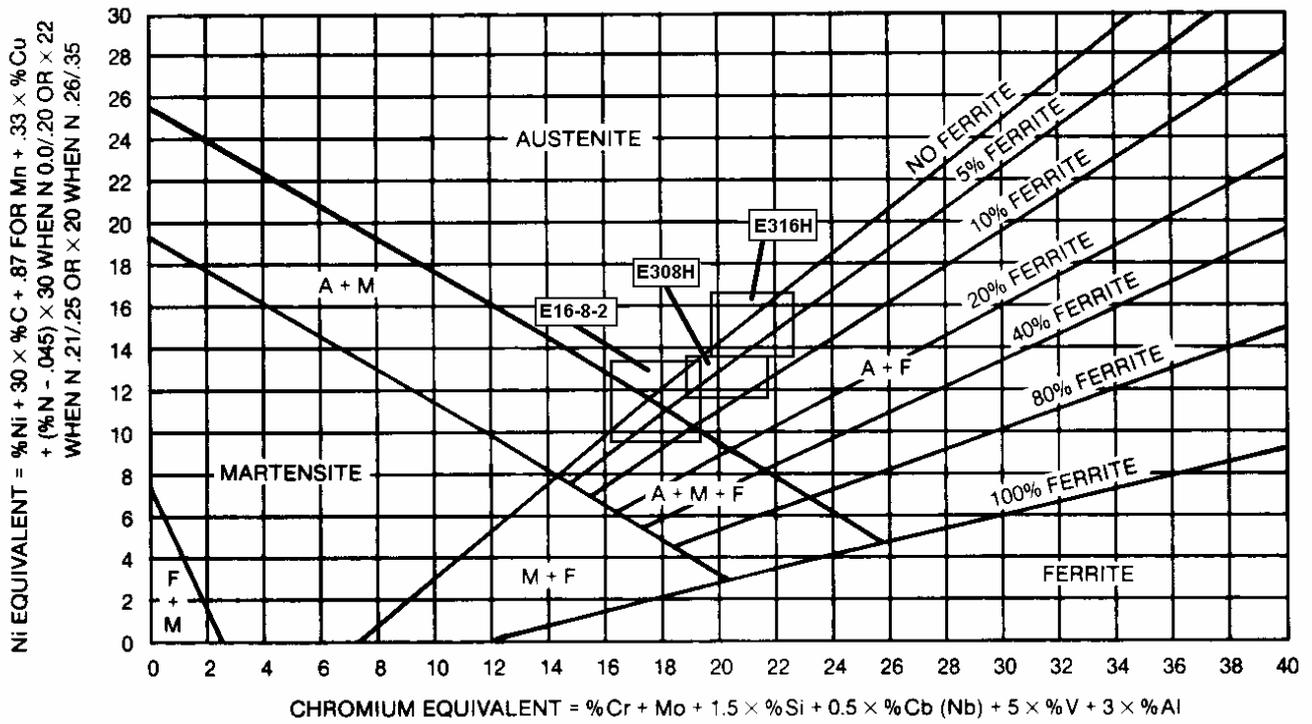
Figure 1: Espy diagram showing location of 16.8.2 with partially constrained composition limits (see text) and similarly constrained E308H and E316H
