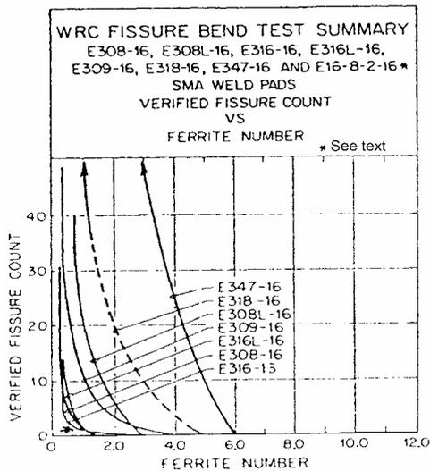
Figure 4: Comparison of the fissuring relationship for eight different austenitic stainless steel weld metals [8,9] Note: E16-8-2-16 showed trivial fissuring and is therefore not plotted
