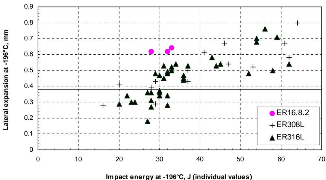
Figure 6: Relationship between Charpy impact energy and lateral expansion of ER16.8.2, ER308L and ER316L SAW weld metals at -196 °C
