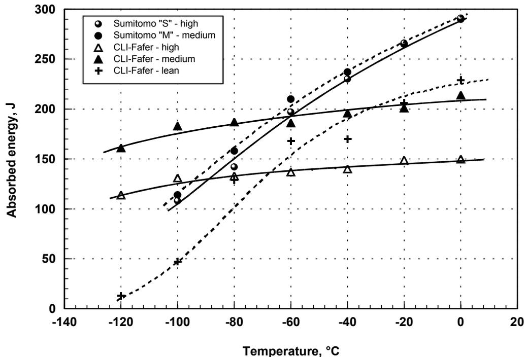
Figure 21. Impact/transition temperature curves plotted from published data from two suppliers for various supermartensitic grades of steel.
