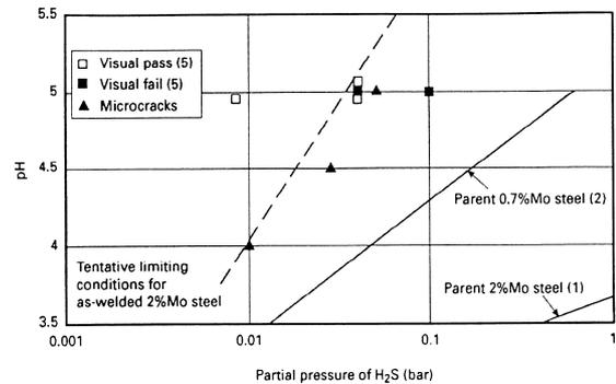
Figure 30: SSC test results and proposed limiting conditions for weldments in 13%Cr-6%Ni-2%Mo-0.1%Ti using superduplex and type 625 filler metal. Indications were at the toe/HAZ region [92]
