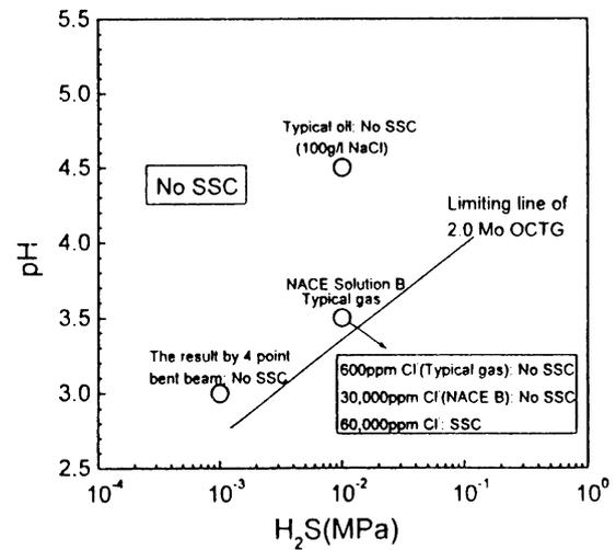
Figure 29c: Effect of H<sub>2</sub>S partial pressure and pH on SSC resistance of the welded joint in Steel 13Cr-S (Cyclic SSRT, 25°C, 5%NaCl) [90]
