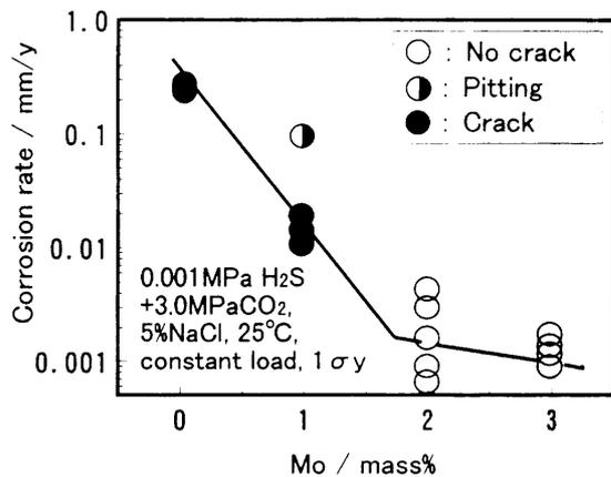
Figure 27: Effect of Mo content on corrosion rate and SSC susceptibility [54].
