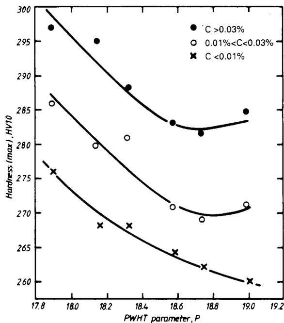
Figure 18: relationship between average weld metal hardness levels (maximum value for each weld) and PWHT parameter,  $P = T(20 + \log t) \times 10^{-3}$ ; hardness data divided in terms of deposit carbon content [29].
