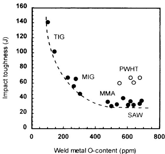
Figure 25: Dependence of Charpy-V impact toughness at  $-40^{\circ}\text{C}$  of Mo-alloyed supermartensitic weld metals on oxygen content and PWHT [11].
