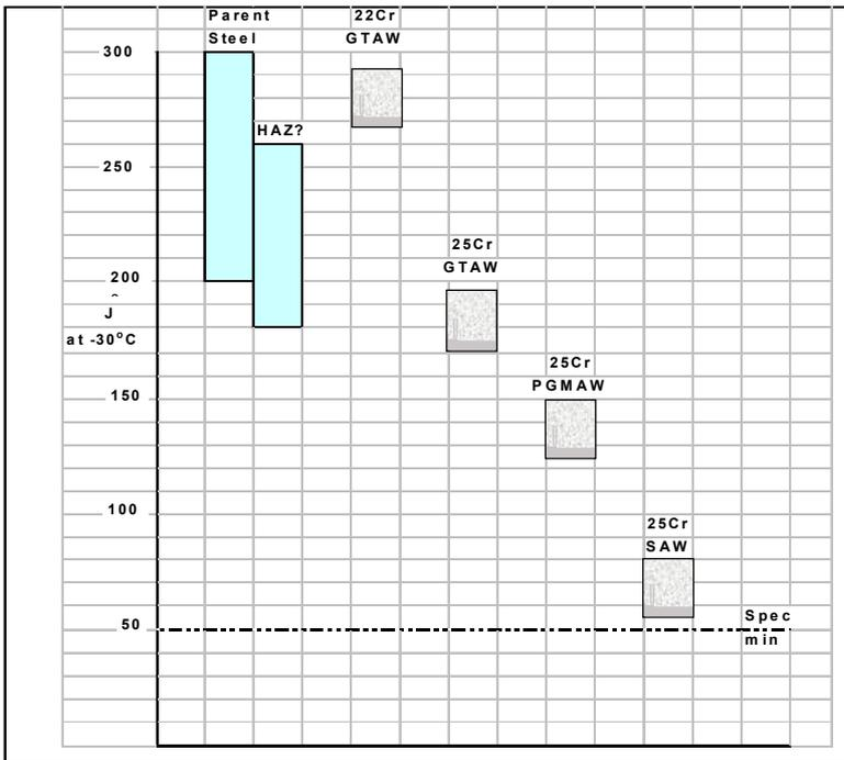
Figure 24: Typical impact values at  $-30^{\circ}\text{C}$  for supermartensitic parent material and HAZ shown in comparison with 25%Cr and 22%Cr duplex weld metals from a number of processes.
