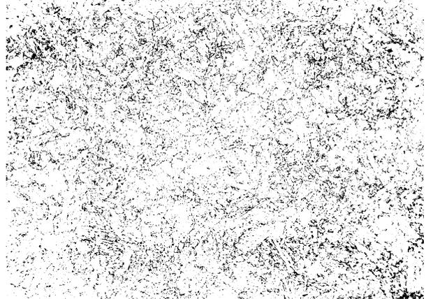
Figure 19 Microstructure of 0.01%C-12.6%Cr-6.4%Ni-2.1%Mo supermartensitic steel. x200
