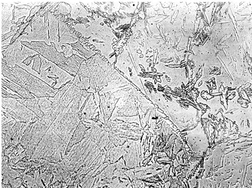
Figure 22: Weld fusion line and HAZ of a supermartensitic steel welded with 25%Cr superduplex filler metal x500
