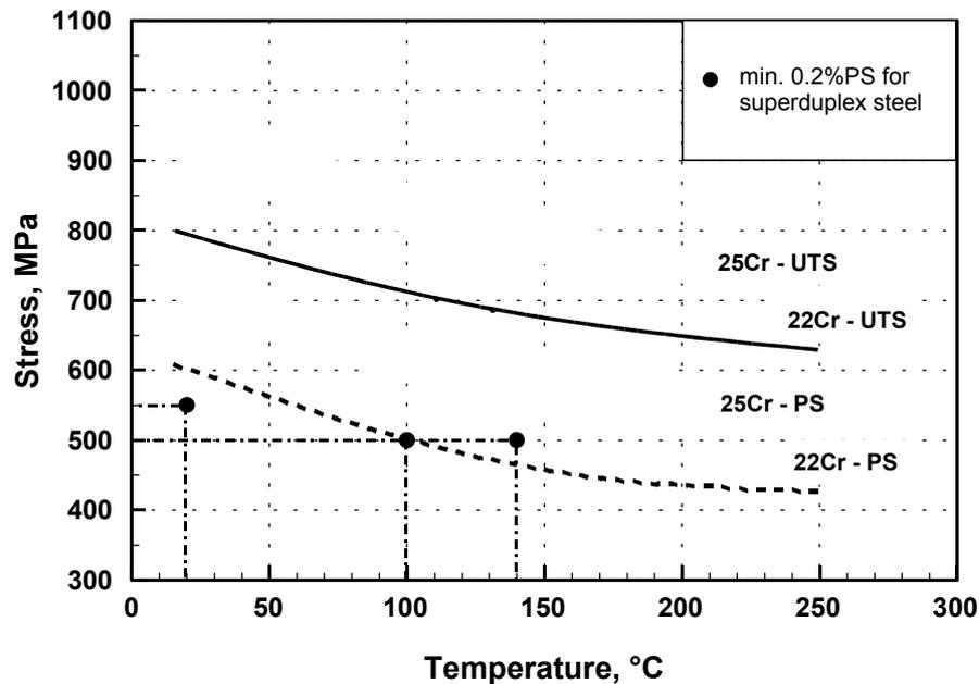
Figure 23. Typical elevated temperature tensile properties for 25%Cr superduplex and 22%Cr duplex stainless steel weld metals together with minimum specified proof stress for superduplex parent steel at elevated temperature.
