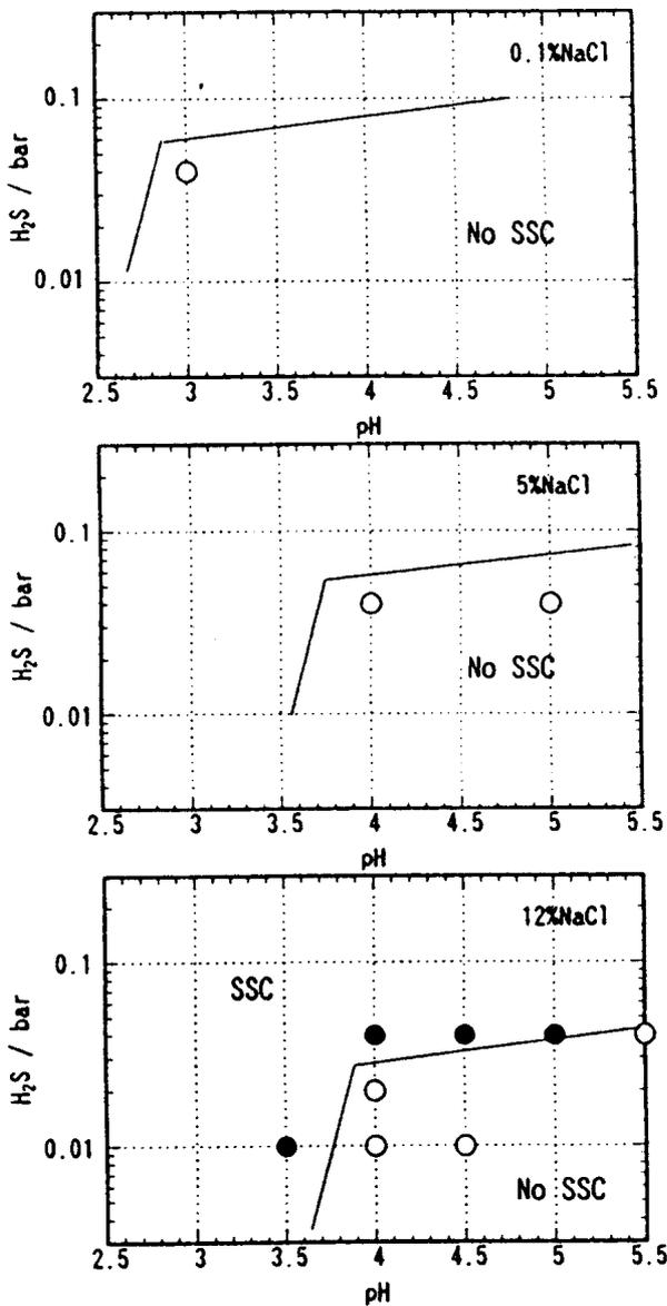
Fig 29b: Effects of Cl<sup>-</sup>, pH and ppH<sub>2</sub>S on SSC occurrence. 2.5PL-M-M, 4-point bent beam, 100%YS, 25°C, 14 days, machined specimen [55]
