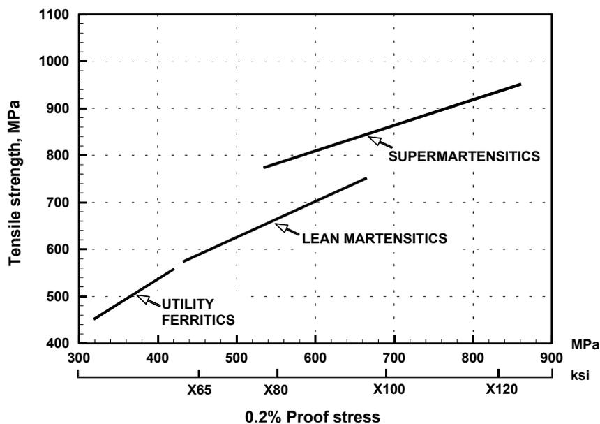
Fig. 20 Tensile strength/proof stress relationship for supermartensitics shown in relation to lean martensitics and utility ferritic steels. Note that the strength of some lean supermartensitics may be close to the lean martensitics.
