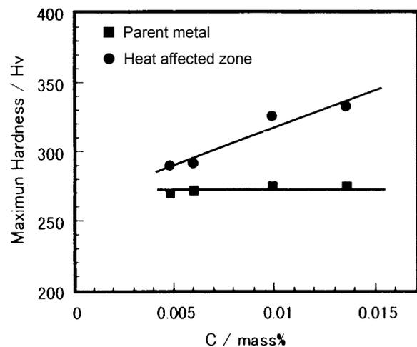
Figure 26: Effect of carbon content on the maximum hardness in parent metal and the heat affected zone [54]
