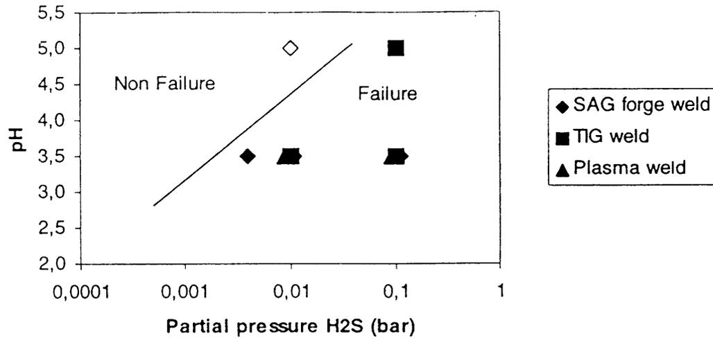
Figure 29a: Environmental limits for welded specimens of super 13%Cr SS tested in buffered NaCl solution at room temperature. Specimens are PWHT at 625°C for 3-10 minutes. Open marks indicate non-failure, while filled marks are registered failures [91]
