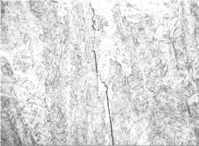
Figure 17: Typical hydrogen crack in martensitic weld metal – note presence of some light etching  $\delta$ -ferrite. x300
